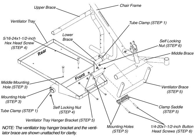
FIGURE 4 - INSTALLING THE VENTILATOR TRAY ONTO THE CHAIR FRAME
